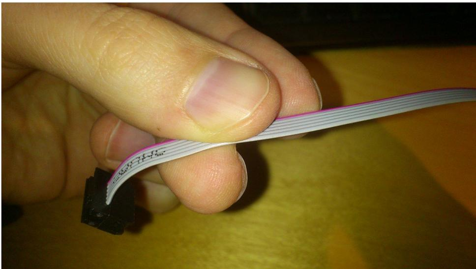
Find the 4<sup>th</sup> wire from the top of the image (counted from the red wire as #1), peel it about 3 mm and solder it to the point marked VGA in the next image. This is just right of the big capacitor on the motherboard:
